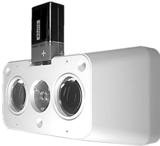
Fig. 2 DOP-6001R detector during optical path alignment
